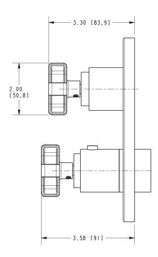
NOTE: Product Dimensions for the Shower System Control Valve Handle Trim (Handle/Escutcheon can be found within the Spec Sheet for that specific part number.
