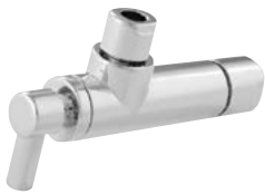
403-1 1/4" Turn Ceramic Disk Angle valve, contemporary style with lever handle. Inlet 1/2" compression. Outlet 3/8" compression.
