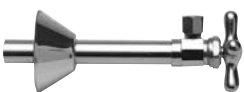
416X Angle Valve with Cross Handle 1/2" sweat x 3/8" O.D. Compression with 11/16" bell flange.
